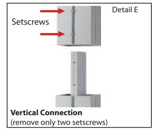
When vertical extrusions are packed in portable cases rather than crates or tubs, they must broken down into smaller sections which then require assembly.
